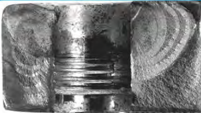
● QF had to account for the complication of tensile crack extensions (darker grey areas) due to peak manoeuvre loads. These show up better optically compared to SEM fractographs
