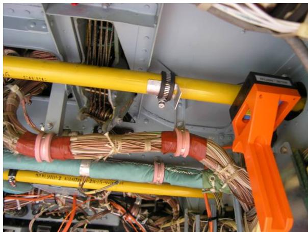
*Figure 2: Non-intrusive laser sensor (on orange bracket) and reflector (on yellow push-pull rod) below cockpit floor to measure stick position*
