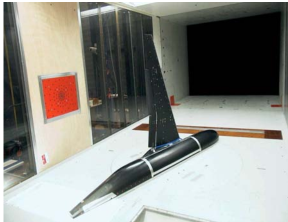
Fig. 6 The model as mounted in the DNW-LST with acoustic array antenna in side-wall
