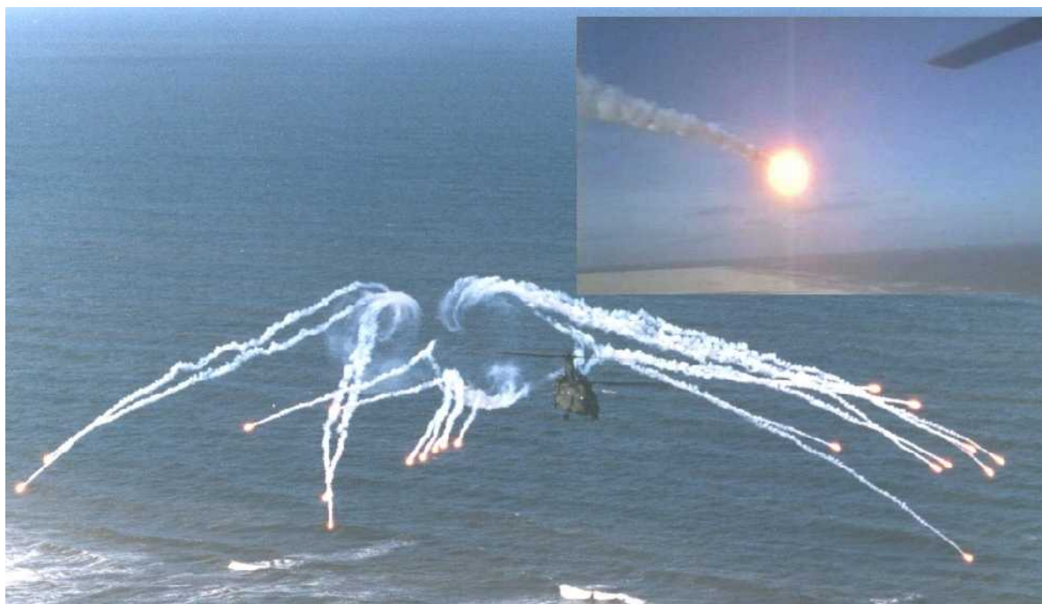
Fig. 2 Flare separation trials on RNLAf CH-47D Chinook (photo: RNLAf)
