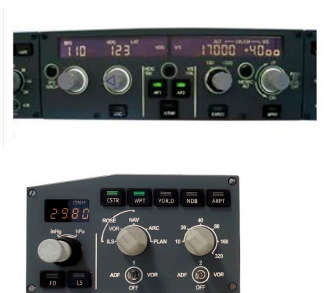
Fig. 3. Top: Airbus Flight Control Unit (FCU) and bottom: left-side EFIS Control Panel.
