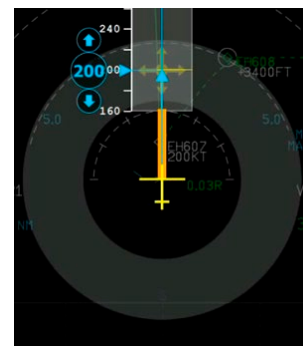
Fig. 11. Setting a new heading (by right pilot)
