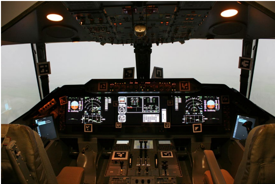
Fig. 20. Touch screens installed inside NLR's full flight simulator (GRACE). Also eye-tracker markings are shown.
