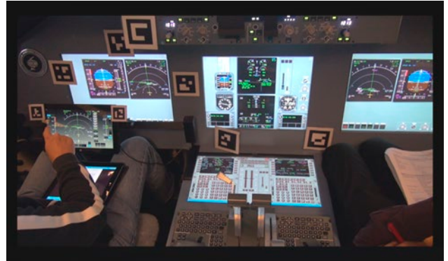
Fig. 2. Tablet touch screen with first HMI-prototype in use inside NLR’s fixed-based flight simulator (APERO). Also eye-tracking reference markers are shown.
