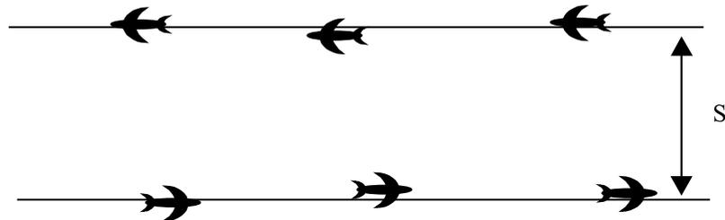
Figure 2 Opposite direction traffic lanes at one flight level
