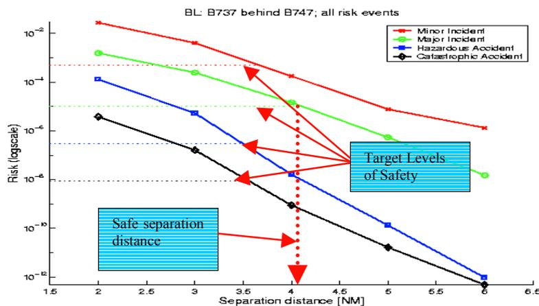
Figure 4: Method to derive safe and appropriate separation minima
