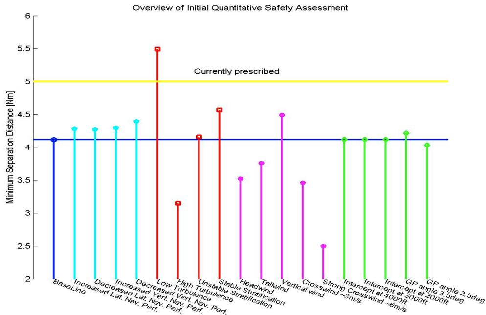
Figure 5: Derived Separation Minima under different operational and weather conditions for a B737 behind a B747.
