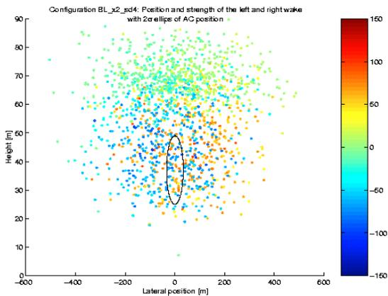
Figure 2: Position and strength data of vortices with 2σ ellipse of the position of the follower aircraft at 5 NM separation
