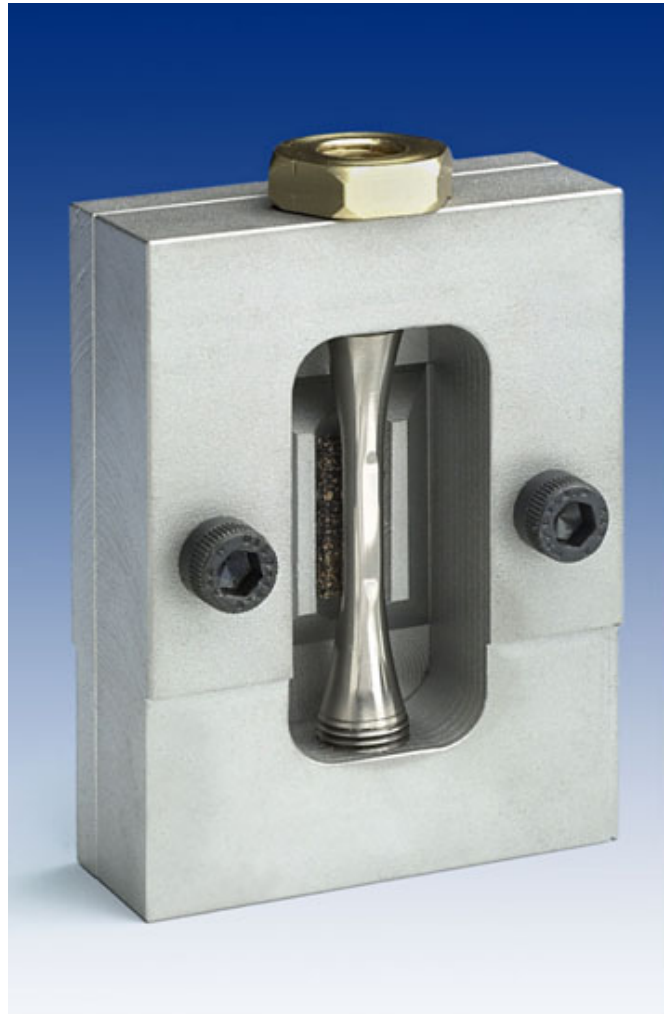
Fig. 3 FOD + HCF specimen in support fixture before impact testing. The back of the specimen is supported by a cork sheet
