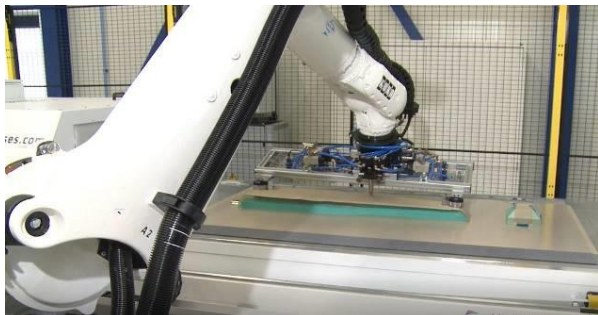
Figure 7: Placing Flat preform on HDF mould
