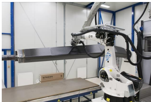
Figure 2: AFP of a 6 meter thermoplastic pylon spar for an engine pylon
