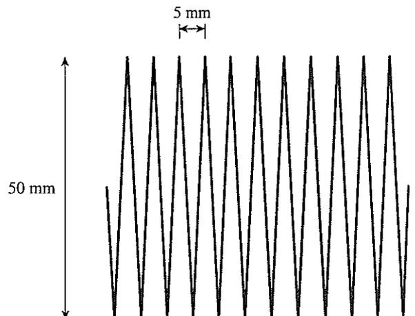
Figure 2: Dimensions of serrated trailing edges
