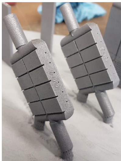
Figure 5 Photo of some samples as they come out of the 3D printer (so before post-processing)
