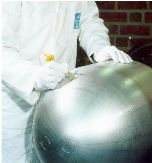
Fig. 2a Installation of a CSA ring on the tank core
