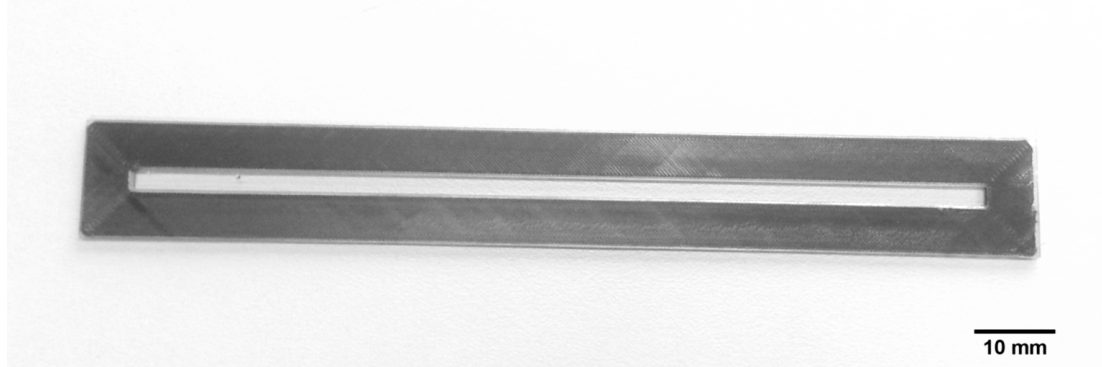
Figure 7: Picture of the printed samples from which the tensile, bending and compression coupons are extracted. The thickness is 2 mm and the final width of the coupons is 15 mm.
