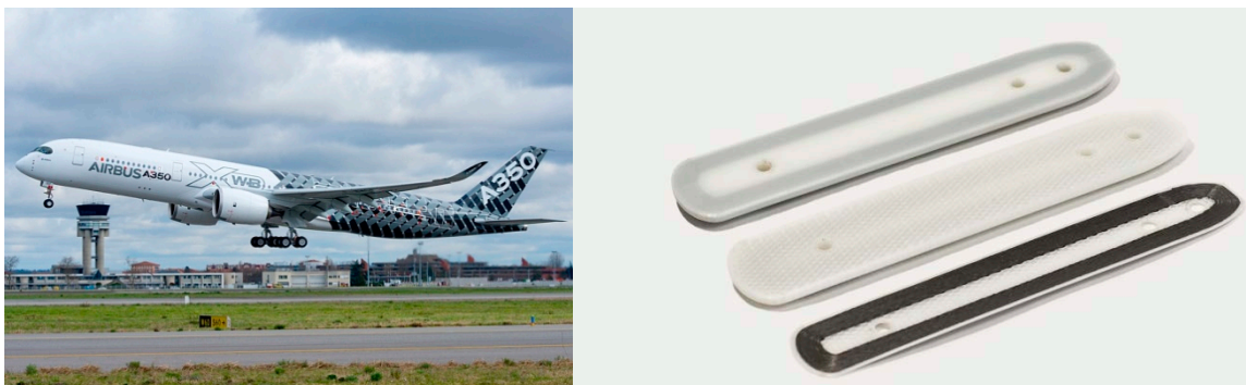
Figure 1: On the left the Airbus A350 for which main components are constructed from carbon fibre reinforced material (source: Airbus). On the right 3D printed examples reinforced with carbon fibres in the contour (source: MarkForged)
