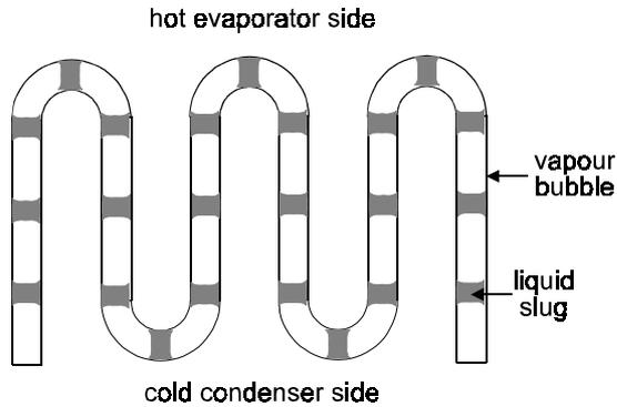
Figure 14. Schematic of an oscillating device section
