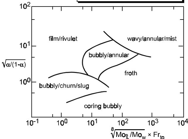
Figure 2. Flow pattern map (vertical downward flow)
