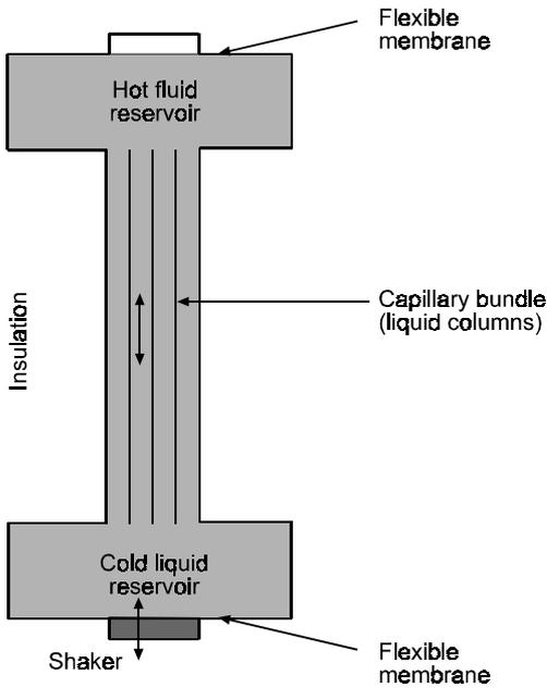
**Figure 11. Synchronised forced oscillatory flow heat transfer device**
