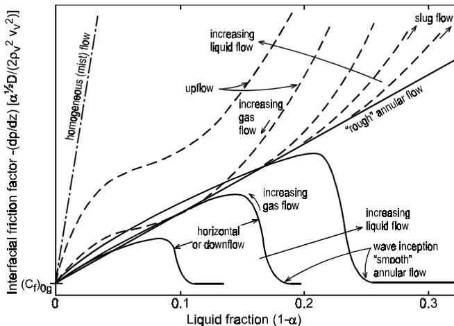
**Figure 9. Qualitative aspects of pressure gradient (apparent friction factor) for various flow patterns**
