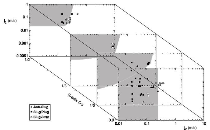
Figure 8. Slug/plug flow: Gravity dependent 3-D map
