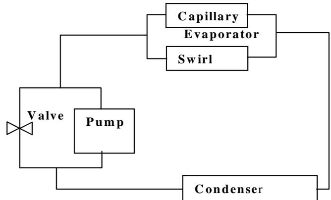
Figure 1. Two-phase loop layout
