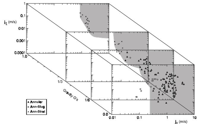
Figure 7. Annular flow: Gravity dependent 3-D map
