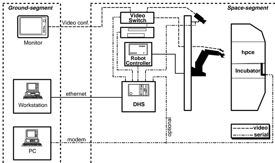
(Figure 6 - Telerobotics system configuration)
