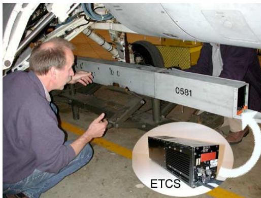
Fig. 9. Mounting of the centreline pylon with ETCS.
