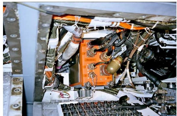
Fig. 10. ETRG installed in aft avionics compartment.
