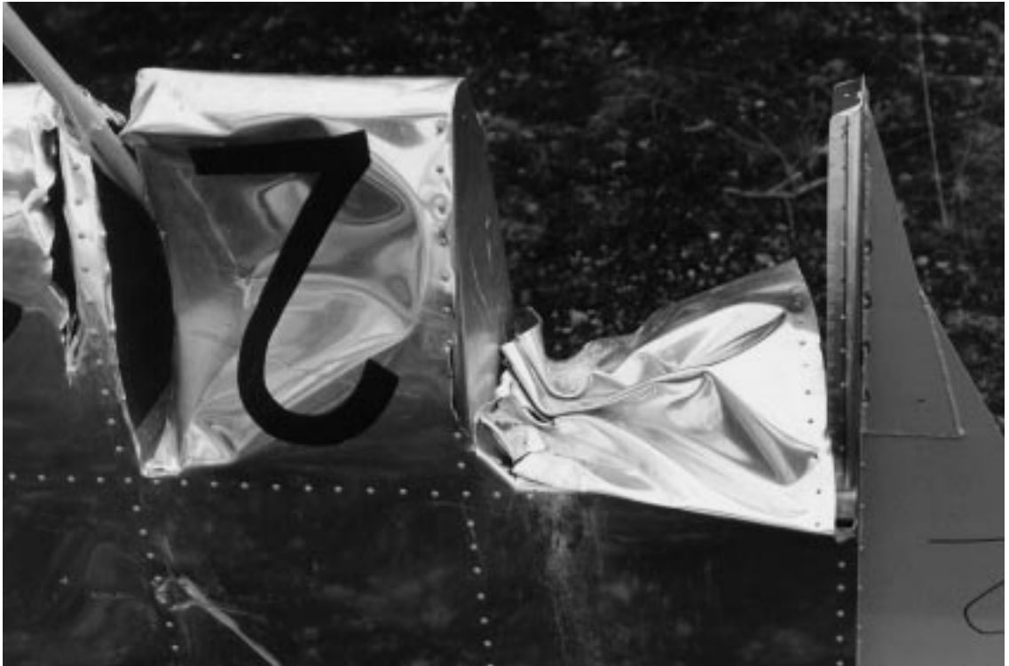
Figure 4. Damaged wing impactor
