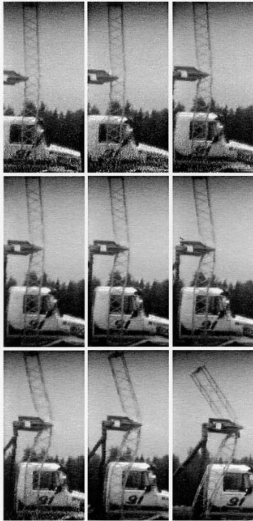
Figure 3. Nine stages of the full scale test on a EXEL mast, test 1 [Ref. 1]
