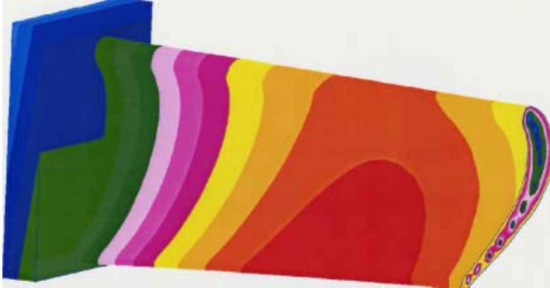
Fig. 8 Computed temperature distributions in gas turbine blade including cooling channels
