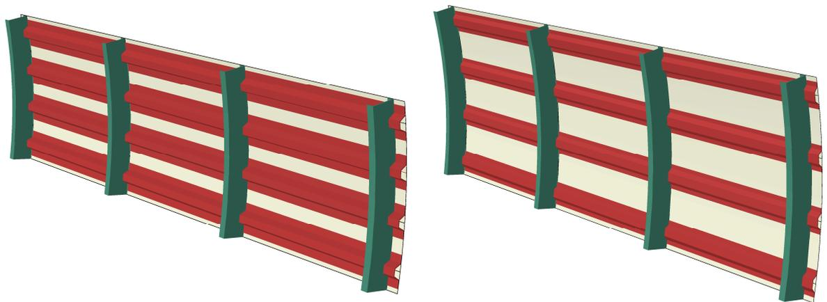
Figure 1 Initial (left) and optimal (right) fuselage panel design
