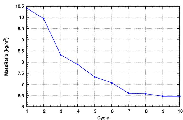
Figure 2 Mass ratio optimisation history for the fuselage panel
