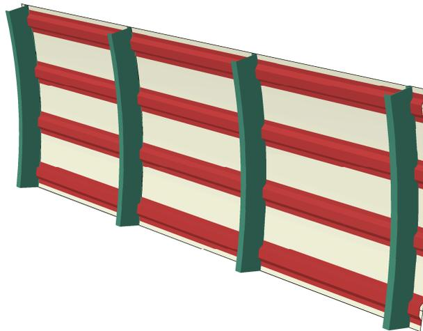
Figure 4 RBO optimal fuselage panel design
