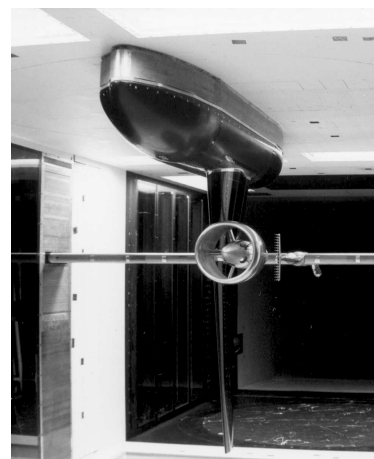
Fig 2 ALVAST Body Wing Through Flow Nacelle half-model configuration in DNW-LST
