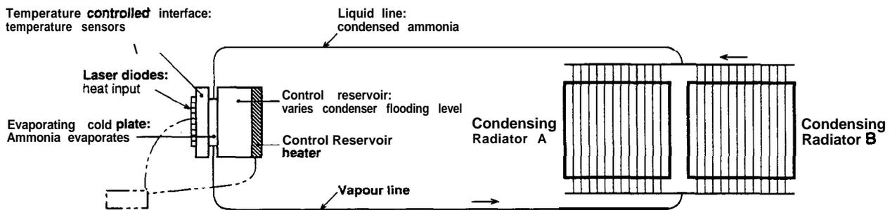
FIGURE 8. ATLID Laser Head Thermal Control Schematic.
