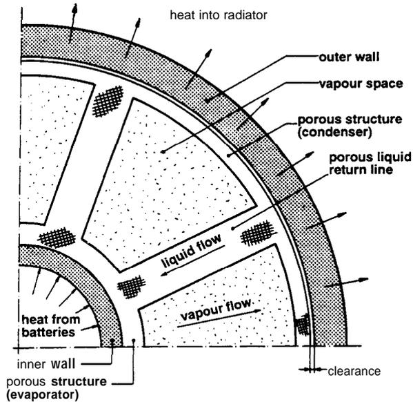
FIGURE 1. Cross-section of a Radial Heat Pipe Joint.
