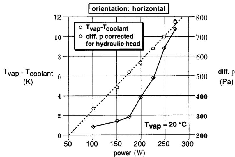
FIGURE 10. Temperature and Pressure Drops as a Function of Power for the Horizontal Condenser.
