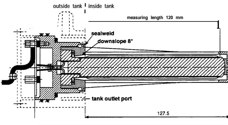
FIGURE 11. Propellant Gauging Sensor Unit.
