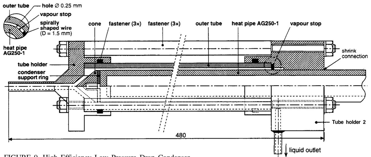
FIGURE 9. High Efficiency Low Pressure Drop Condenser.
