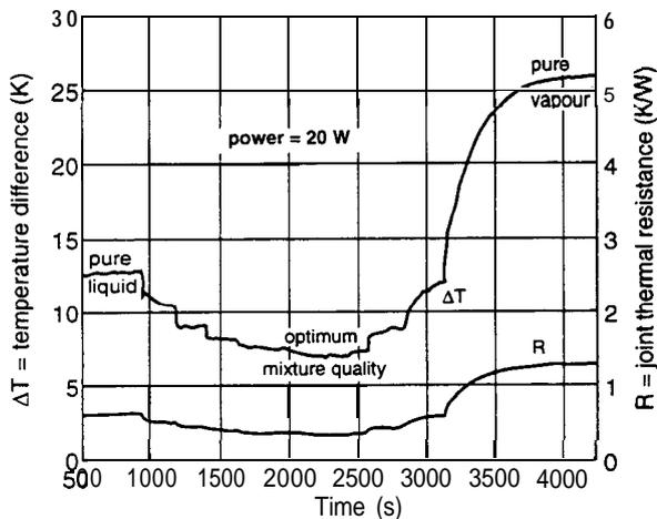
FIGURE 3. Determination of Optimum Filling.
