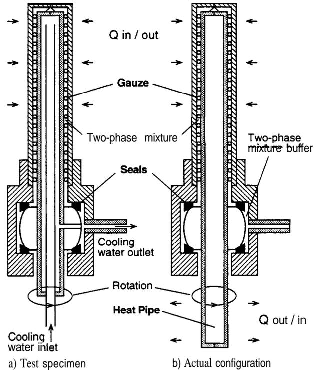
FIGURE 2. Rotatable Radial Heat Pipe Joint.
