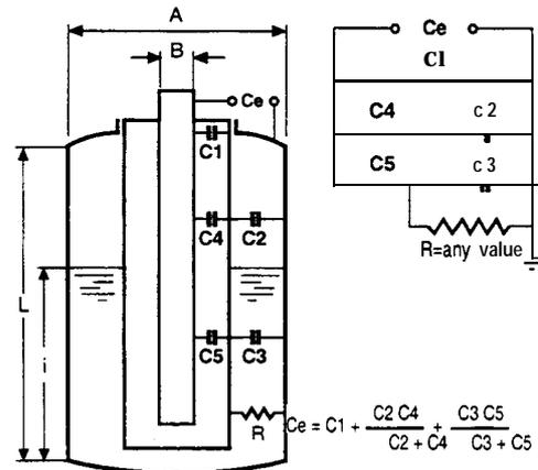
FIGURE 12. Coated Capacitance Probe (Schematic).
