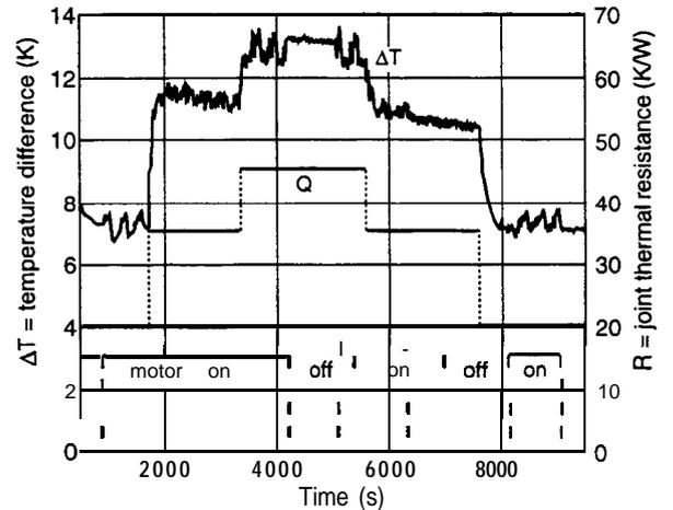
FIGURE 4. Power Dependence of Joint Resistance (non-rotating and rotating at 17.5 rpm).
