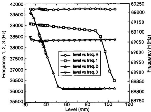
FIGURE 13. GSU Levels versus Frequency Test Data (MON-1).
