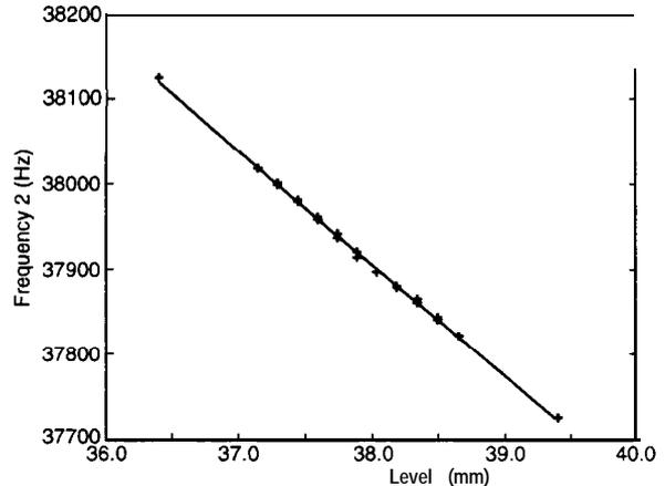
FIGURE 14. GSU Resolution Test Data (MON-I).
