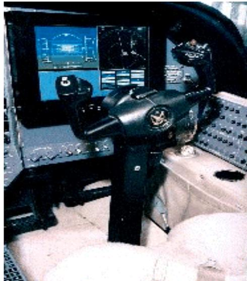
*Figure 2: Primary Flight Display and controls for the Experimental Pilot Flying (PFD EPF)*
