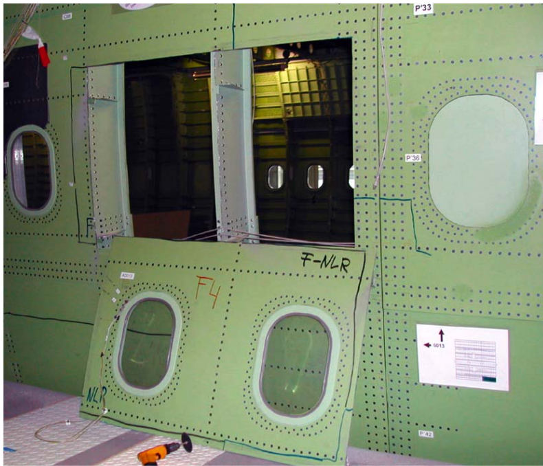
Figure 1 GLARE window area cut from the MLB
