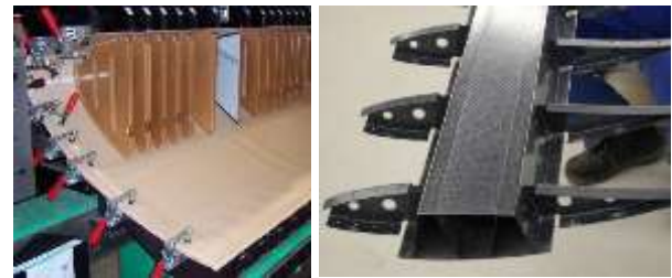
A380 leading edge rib Ribs on the AW169 Figure 6: Examples of press formed parts in aircraft produced by Fokker
