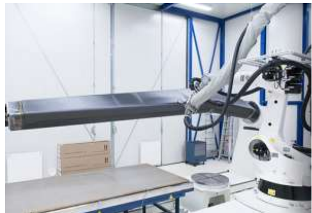
Figure 5: Flat lay-up concept for skin preforms with NLR's AFP machine (top); NLR's AFP machine placing a large thermoplastic pylon upper spar (bottom)
