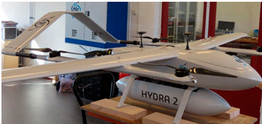
Hydra-2, NLR's hydrogen propelled flight platform. The bottom fairing contains the storage compartment holding the hydrogen tank
