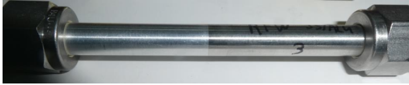
Fig. 5 Example of bi-metal welded joints that could be used to join stainless steel tubing to aluminum vessel. Image - Royal NLR.
