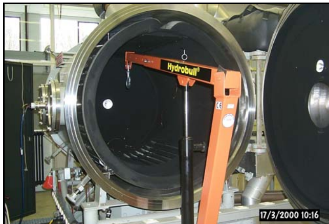
Figure 2: NLR Thermal Vacuum Space Simulator.
