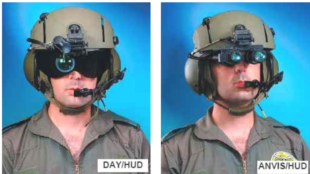
Figure 1: Day (left) and Night Eye HUD of the ESL ANVIS/HUD-24 system
