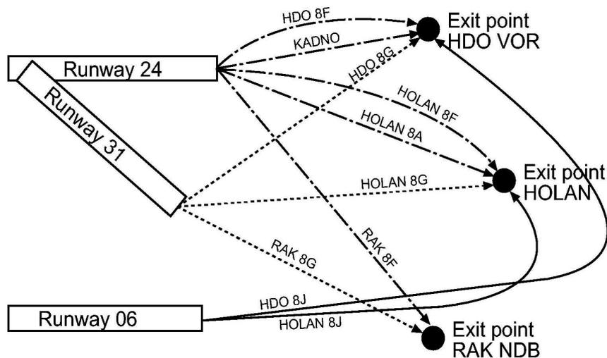
*Fig. 1. Schematic representation of part of Prague airport: runways, SID routes, exit points*
