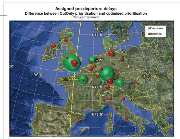
Figure 6. Geographical distribution of differences in assigned pre-departure delays at airports between OutOnly prioritisation and optimised prioritisation for the reduced+ scenario
