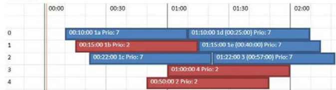
Figure 4 - Example of making a reservation for a prioritised flight during a condition of overload
