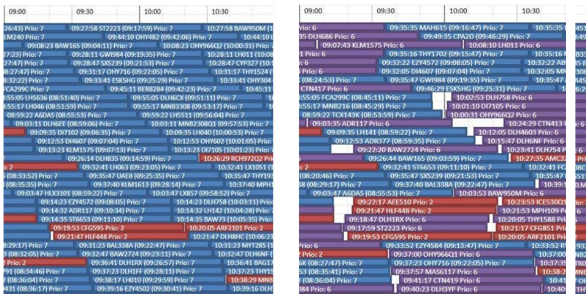
Figure 11- Example showing difference in allocation of reservations at EDMMUR3, using OutOnly and MainHigher prioritisation
