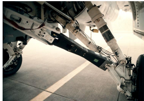
Figure 10: Composite drag brace after assembly in the F-16 main landing gear
