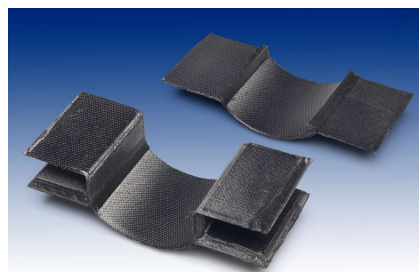
Figure 6: Net-shaped preforms for the lug area of the trailing arm using binder technique.
