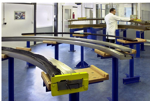
Figure 12: RTM carousel showing two preform tools and the oil heated outer RTM tool.
