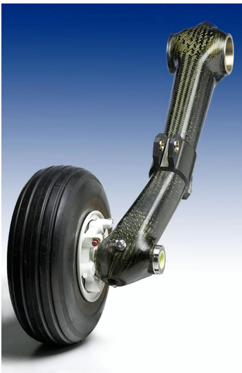
Figure 7: Composite trailing arm after assembly
