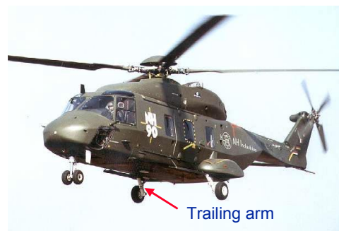
Figure 3: Location of the trailing arm in the main landing gear.
