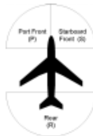
Fig. 4 Lateral airspace segments, for Extended VFR Overtaking rules
