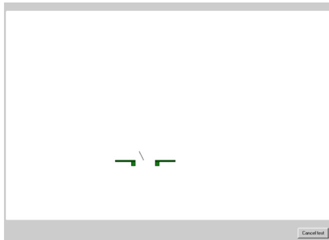
Figure 2: Example screen layout as used for the tracking task. The participant could control a tracking symbol ('bucket') by using a one-dimensional joystick. The task was to keep the small line segment centred above the bucket. Due to the size of the small line segment, almost no preview was present in this tracking task.
