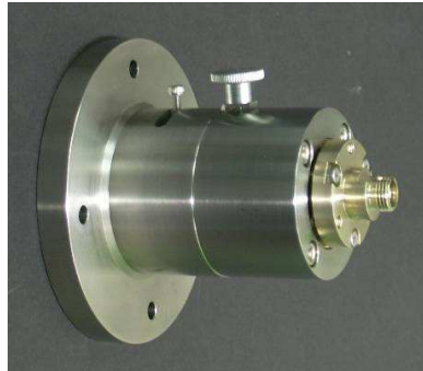
Figure 4 The optical head of which four are installed in the aircraft.
