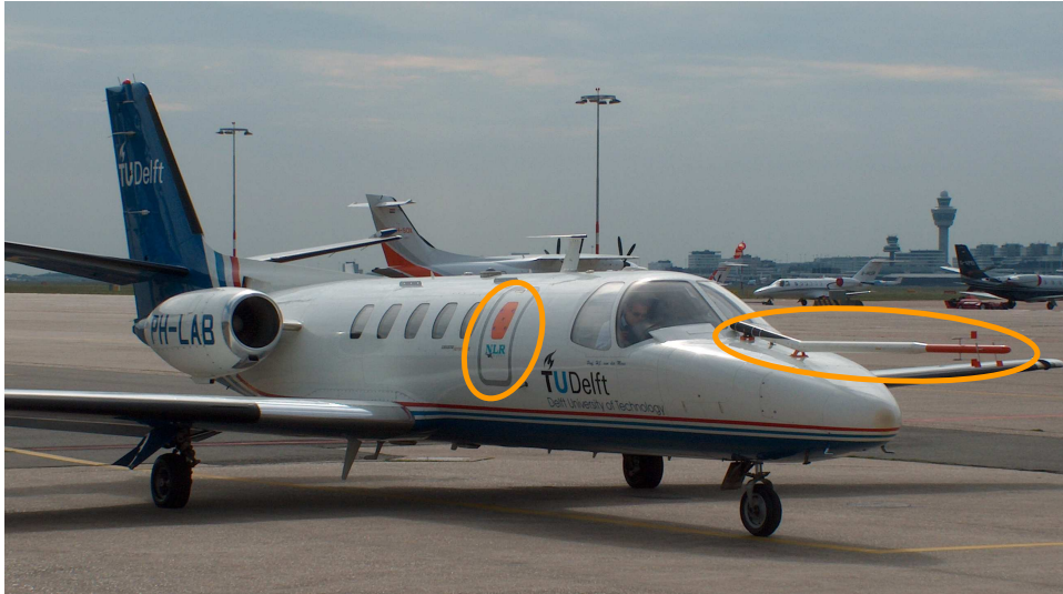
Figure 1 NLR's Cessna Citation II research aircraft ready for a NESLIE test flight from Amsterdam Airport Schiphol with the modified emergency hatch and noseboom.
