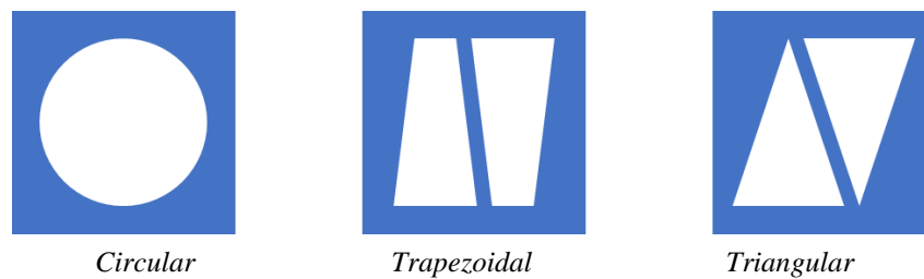
Figure 2. Channel geometries for parallel channels under consideration
