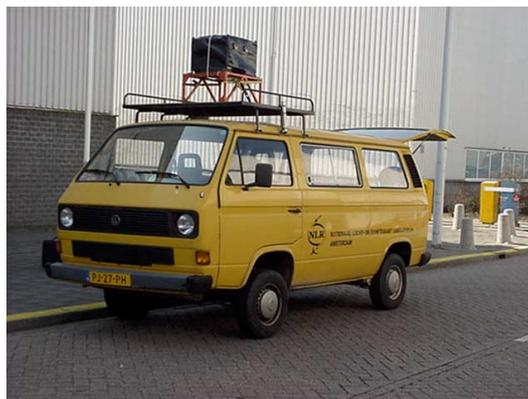
*Fig. 2 Spades control unit installed on a van for a simulated flight on the earth*
