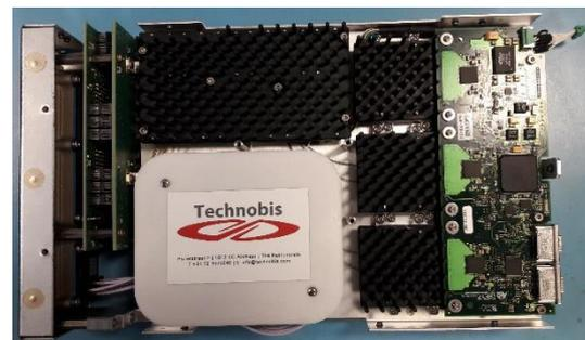
**Figure 5.** Optical part FOPU prototype with 6-channel FBG interrogator fitted with heat sinks from PhotonFirst (known as Technobis Fibre Technologies before 2021).
