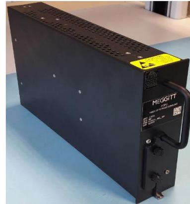
**Figure 4.** FOPU prototype- External view – ARINC 600 2MCU rackable avionic unit.
