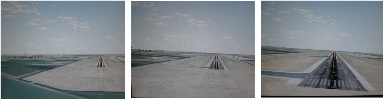
Figure 4. GRACE visual database illustrating the sequence of the outside visual scene during the piloted decrab maneuver for a left crosswind (from left to right).
