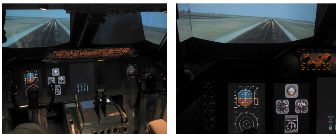
Figure 3. NLR GRACE transport aircraft cockpit for the pilot motion perception and control experiment. Left: GRACE cockpit in Fokker 100 configuration. Right: Left pilot's view on primary instruments and outside scene during the decrab maneuver.
