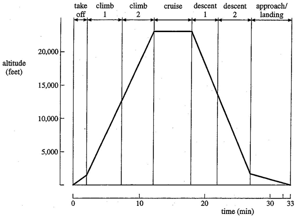
Fig. 1 Mission profile and segments for a short haul transport
