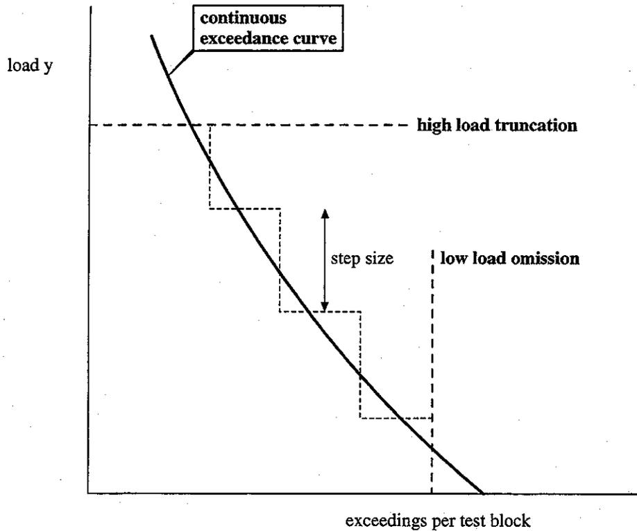
Fig. 2 Stepping of a continuous exceedance curve
