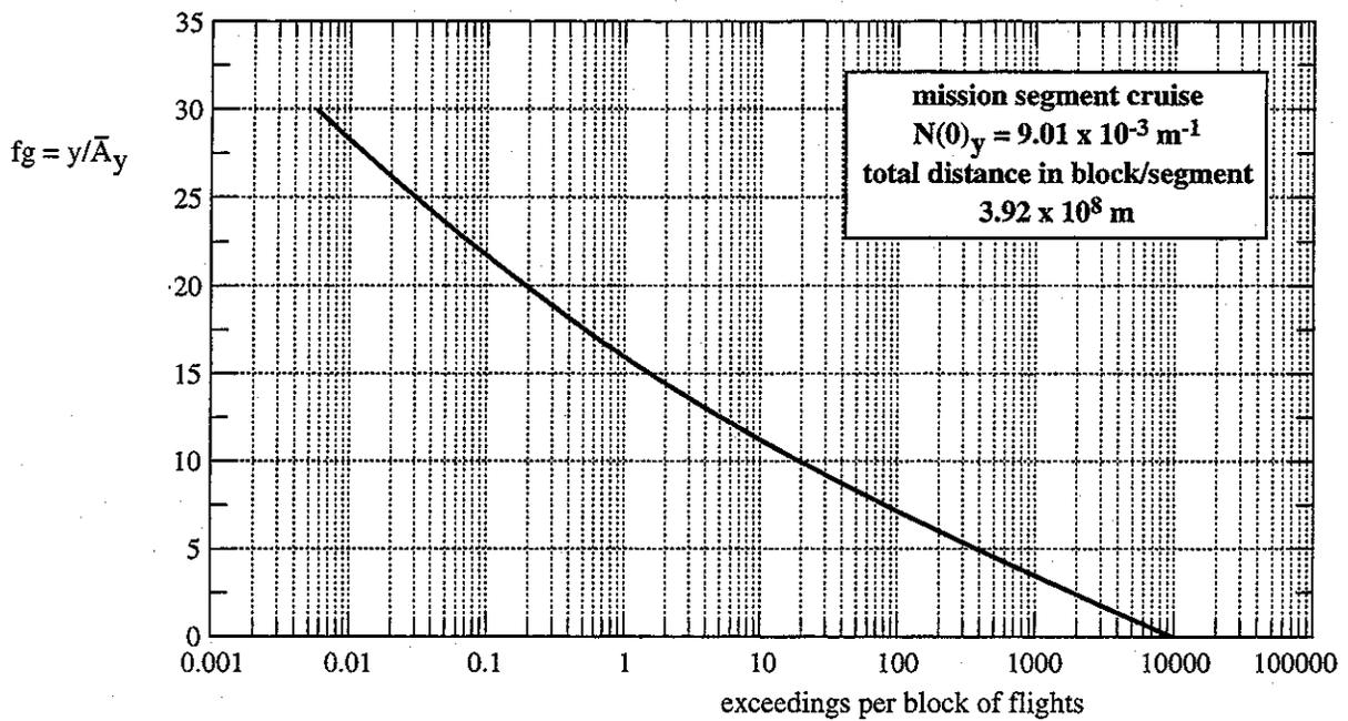
Fig. 6 Exceedance curve for gust strength factor  $f_g$
