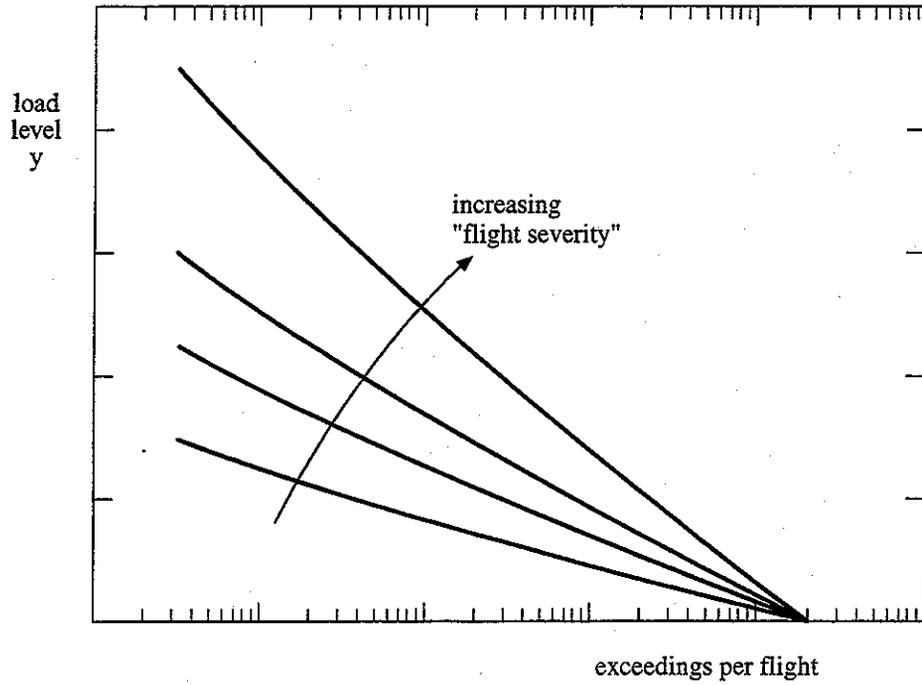
Fig. 3 Flight load spectra with equal shape but different severity
