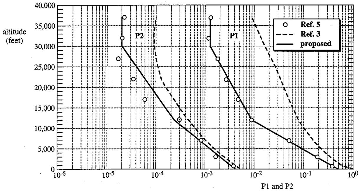
Fig. 4 Proposed P-values for turbulence model
