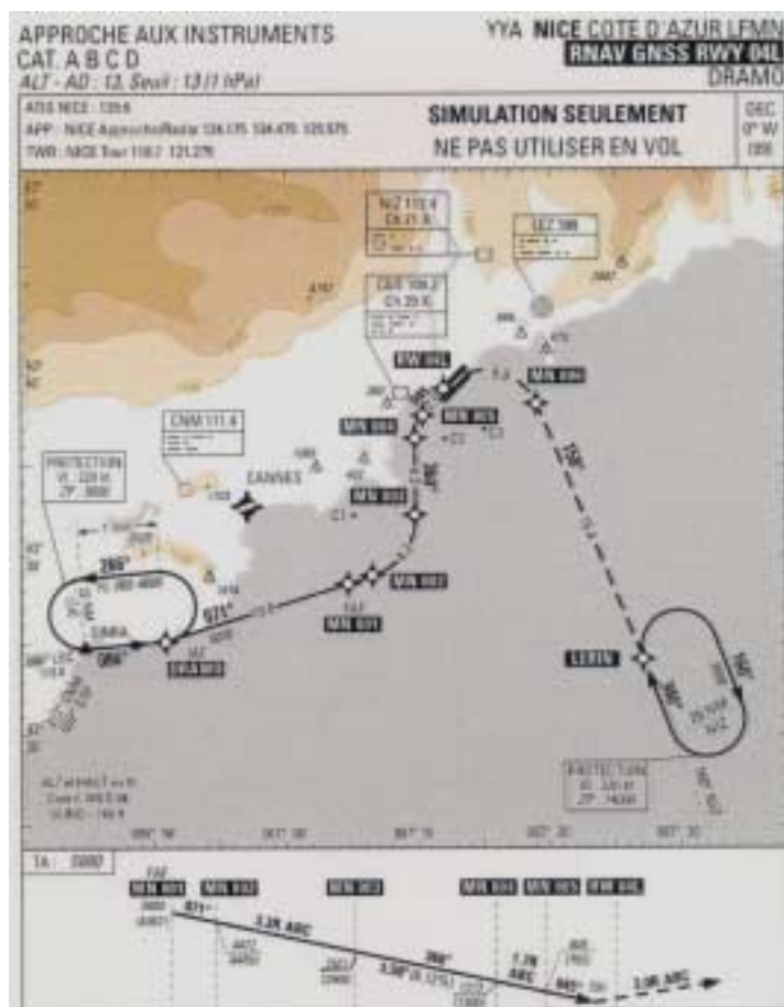
Figure 2 DRAMO Experimental Approach Procedure at Nice airport
