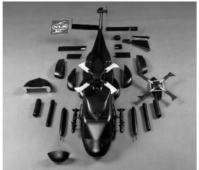
Fig.5: Components of fuselage model (photo: NLR)
