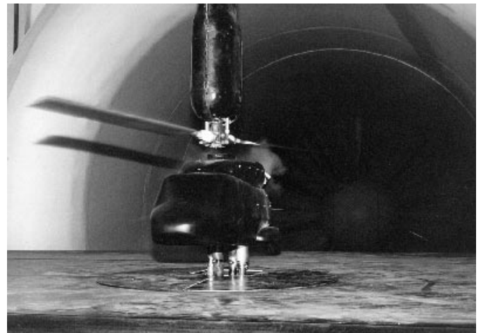
Fig.11: Engine recirculation model in ECF wind tunnel (photo: Eurocopter)
