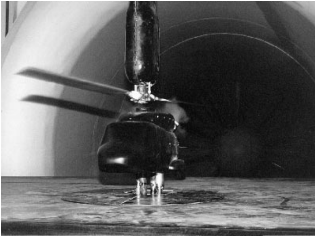
Fig.7: Powered tail rotor model in LST (photo: NLR)
