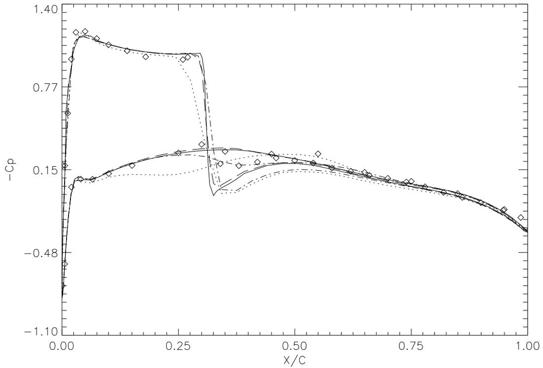
Figure 13: Pressure coefficient  $C_p$  at cross-section  $y = 0.90S$  of ONERA M6 wing,  $M_\infty = 0.84$ ,  $\alpha = 3.06^\circ$  ( $\cdots$  original grid,  $- - -$  one adaptation,  $- - -$  two adaptations,  $- - -$  three adaptations,  $\diamond \diamond$  experiment).
