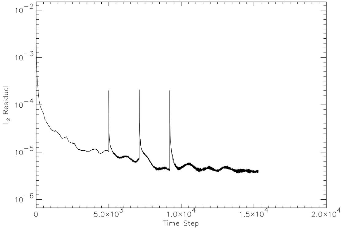
Figure 6: Convergence history of  $L_2$  residual for flow field about ONERA M6 wing.
