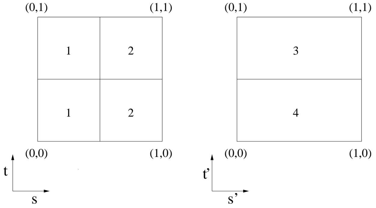
Figure 3: Faces of elements 1 and 2 are split into sub-faces such that each sub-face connects to one element at each side.
