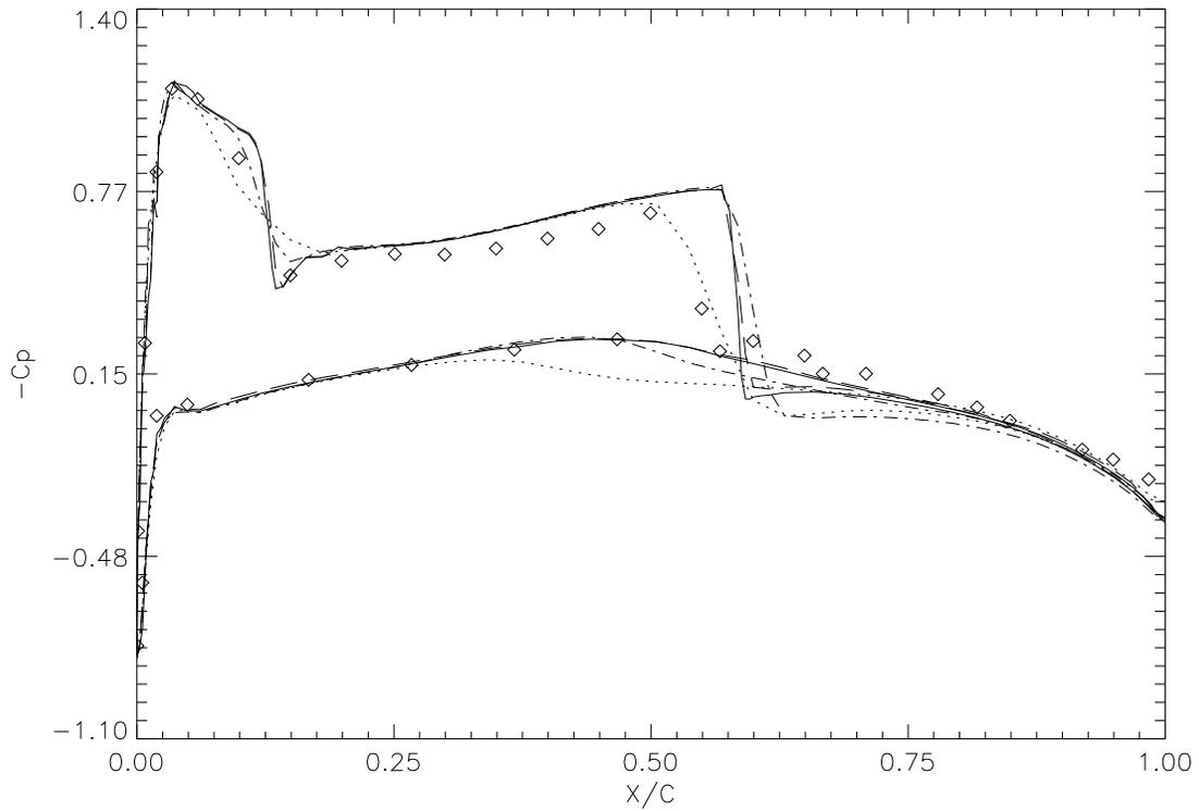
Figure 10: Pressure coefficient  $C_p$  at cross-section  $y = 0.44S$  of ONERA M6 wing,  $M_\infty = 0.84$ ,  $\alpha = 3.06^\circ$  ( $\cdots$  original grid,  $- - -$  one adaptation,  $- - -$  two adaptations,  $- - -$  three adaptations,  $\diamond \diamond$  experiment).
