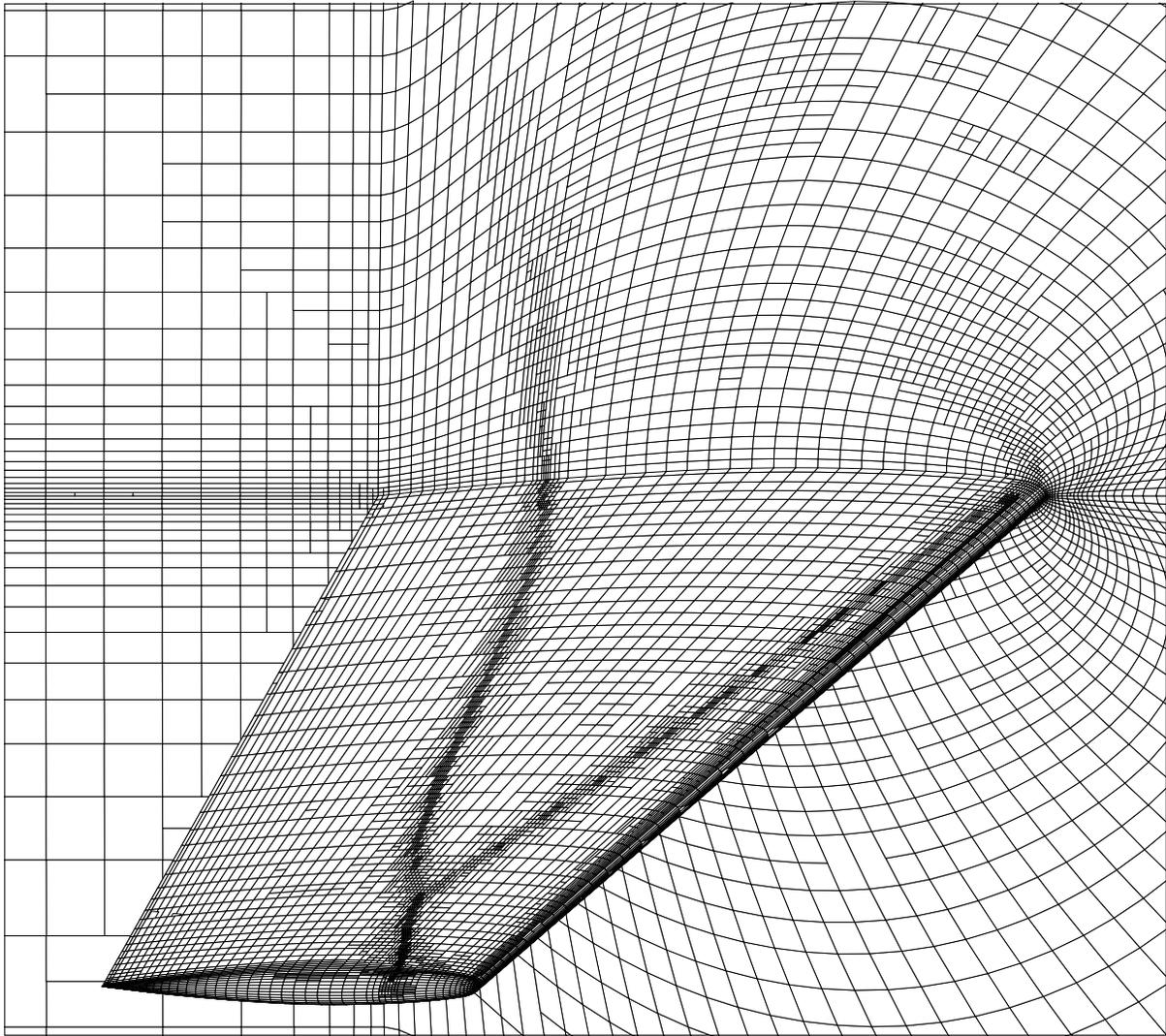
Figure 8: Final adapted grid on ONERA M6 wing,  $M_\infty = 0.84$ ,  $\alpha = 3.06^\circ$ .
