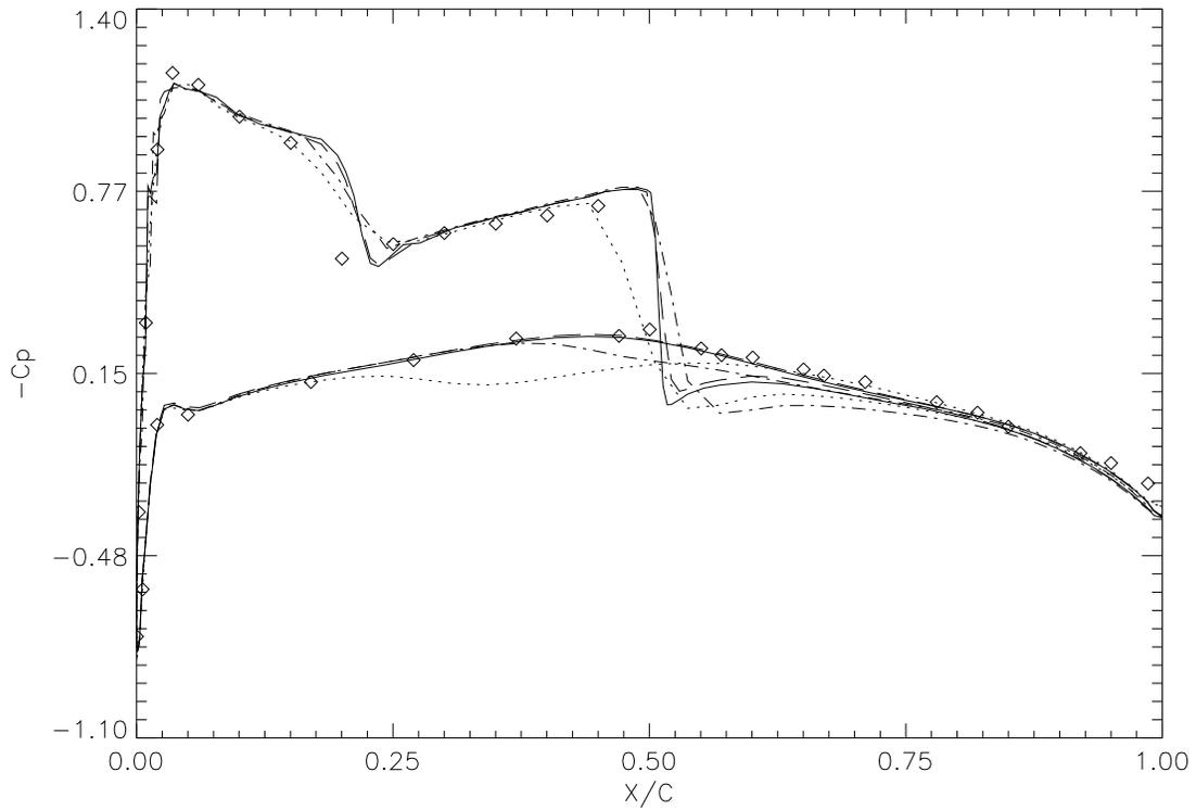
Figure 11: Pressure coefficient  $C_p$  at cross-section  $y = 0.65S$  of ONERA M6 wing,  $M_\infty = 0.84$ ,  $\alpha = 3.06^\circ$  ( $\cdots$  original grid,  $- \cdot -$  one adaptation,  $- - -$  two adaptations,  $—$  three adaptations,  $\diamond$   $\diamond$  experiment).
