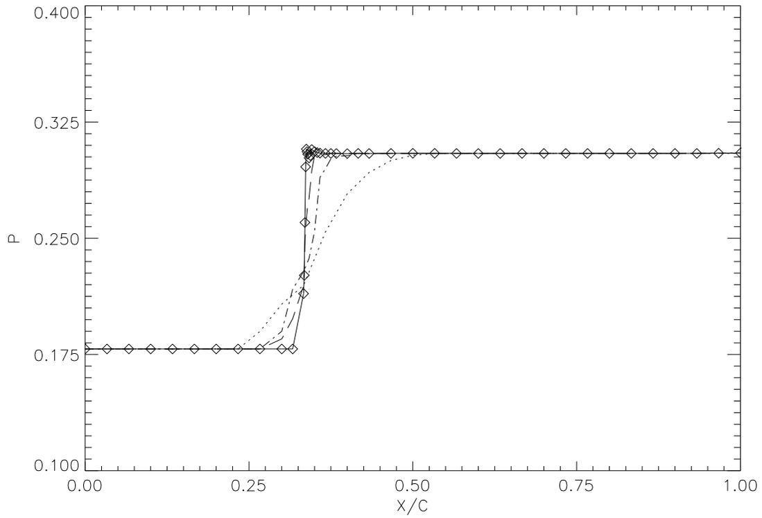
Figure 5: Pressure distribution along a  $10^\circ$  ramp for supersonic flow,  $M_\infty = 2.0$  ( $\cdots$  original grid,  $-\ -$  two adaptations,  $- \cdot -$  four adaptations,  $—$  six adaptations,  $\diamond \diamond \diamond$  final adapted grid).
