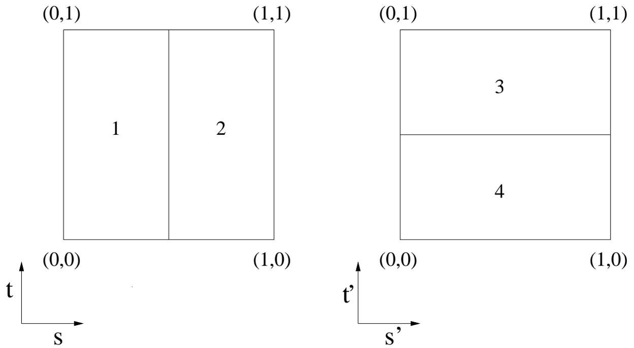
Figure 2: Element refinement at left and right side of elementary face. Elements 1 and 2 can not be connected to elements 3 and 4 with one face.
