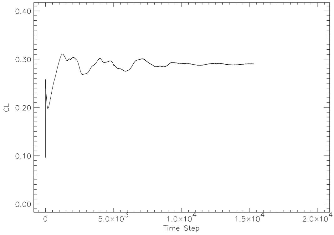
Figure 7: Convergence history of lift force  $C_L$  on ONERA M6 wing.
