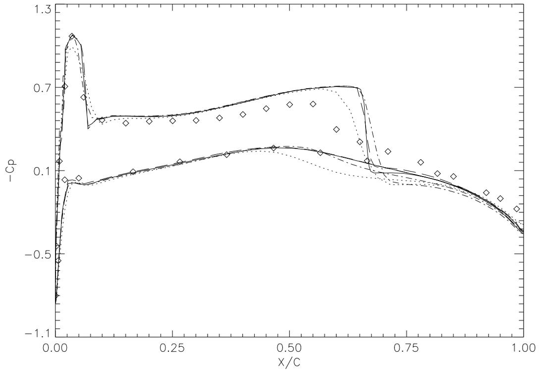
Figure 9: Pressure coefficient  $C_p$  at cross-section  $y = 0.20S$  of ONERA M6 wing,  $M_\infty = 0.84$ ,  $\alpha = 3.06^\circ$  ( $\cdots$  original grid,  $- - -$  one adaptation,  $- - -$  two adaptations,  $- - -$  three adaptations,  $\diamond \diamond$  experiment).
