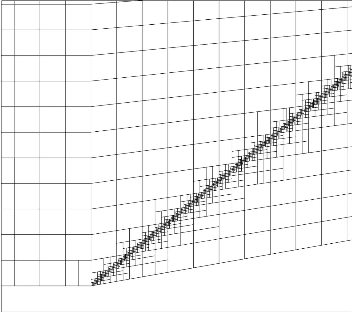
Figure 4: Detail of grid for supersonic flow over a  $10^\circ$  ramp after six adaptations.
