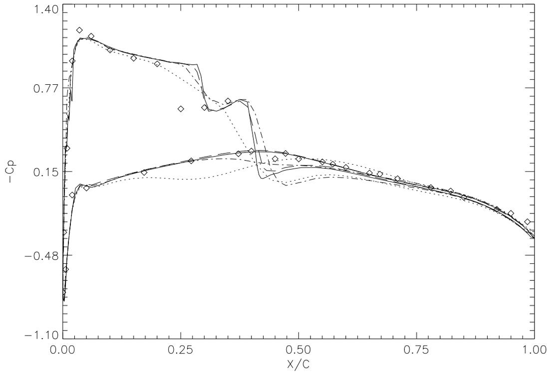
Figure 12: Pressure coefficient  $C_p$  at cross-section  $y = 0.80S$  of ONERA M6 wing,  $M_\infty = 0.84$ ,  $\alpha = 3.06^\circ$  ( $\cdots$  original grid,  $- - -$  one adaptation,  $- - -$  two adaptations,  $---$  three adaptations,  $\diamond \diamond$  experiment).
