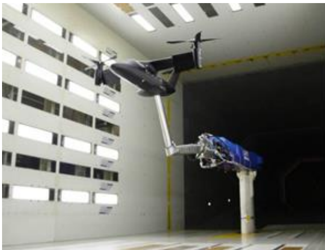
Figure 5: Model on dorsal sting support in DNW-LLF
