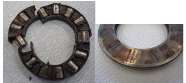
Figure 8: Broken blade axial bearing and damaged bearing ring due to high loads under cyclic blade movement
