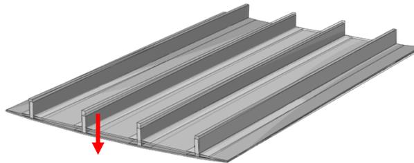
Figure 19: Bending of the rib stiffened panel due to cooling to room temperature after cure
