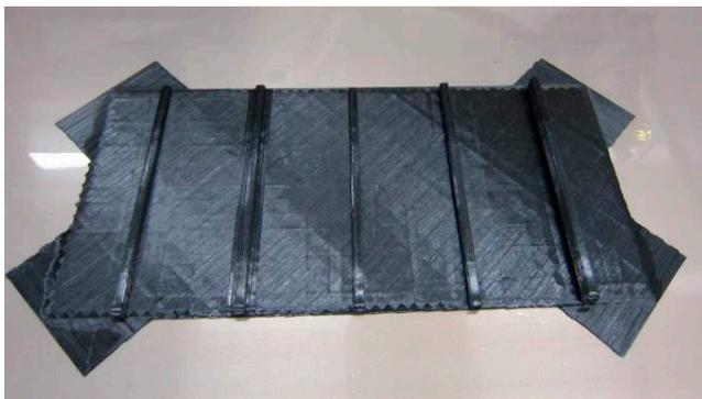
Figure 6: Fibre placed test panel before cure
