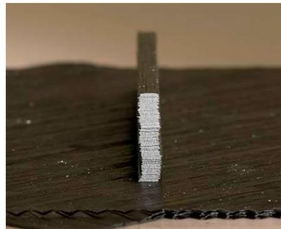
Figure 13: Final result of the rib height trial showing a good quality and stable rib
