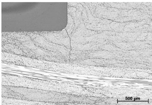
Figure 9: Crack near the corner of rib number 3.
