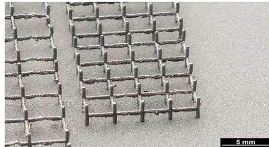
Figure 15: Titanium SLM mesh
