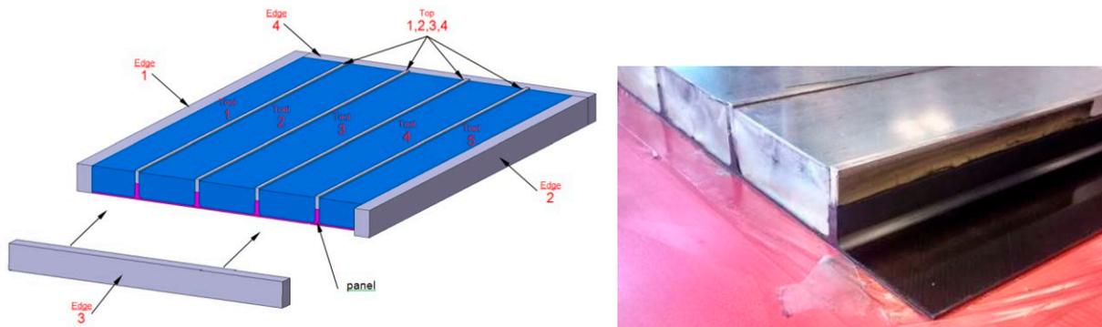
Figure 22: Tooling concept (left) and demoulding
