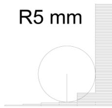
Figure 20: Schematic overview of radius used to "squeeze" tapes into place to form the rib foot
