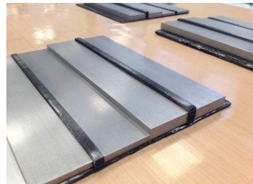
Figure 7: Cure tooling for the manufacturing trials
