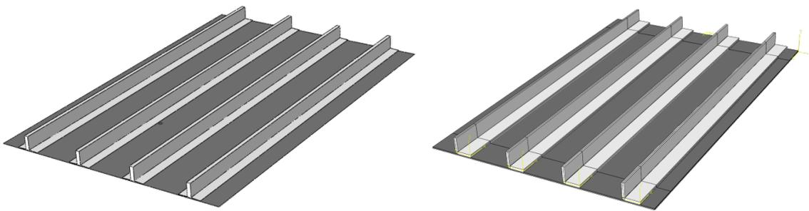
Figure 17: Illustration of the co-cured rib stiffened panel (left) and the co-bonded blade stiffened panel (right)
