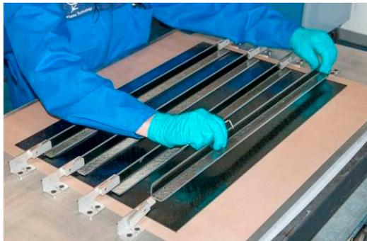
Figure 28: Positioning of stiffeners with grips
