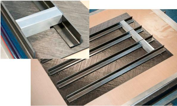
Figure 30: Spacers used to position L-blade stiffeners
