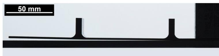
Figure 24: bending due to transversal shrinkage of ribs. Maximum deviation measured 2.7 mm
