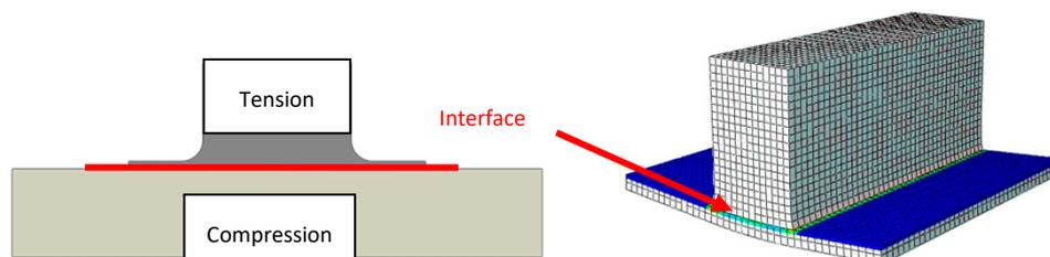
Figure 3: Stress directions after cool down of the co-cured skin and rib part.
