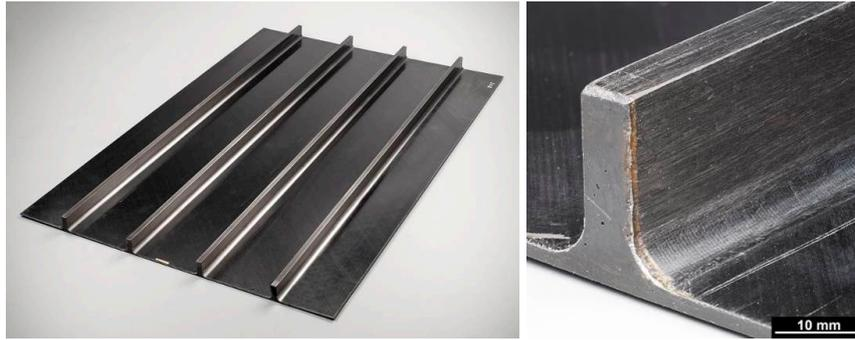
Figure 25: Final rib stiffened co-cured compression panel before machining
