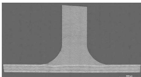
Figure 23: Cross/section of rib stiffener in panel.
