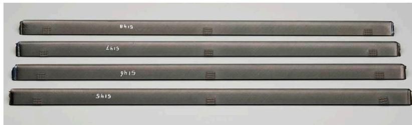
Figure 27: Cured with SLM meshes stiffeners after machining
