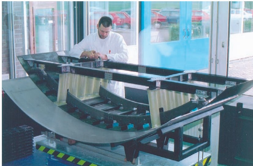
Fig. 8 Final assembly of Commuter sub-floor struct. (NLR)
