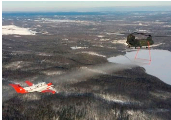
Figure 6. HISS icing spray calibration. RC-12G on station behind the tanker to sample the spray for calibration.
