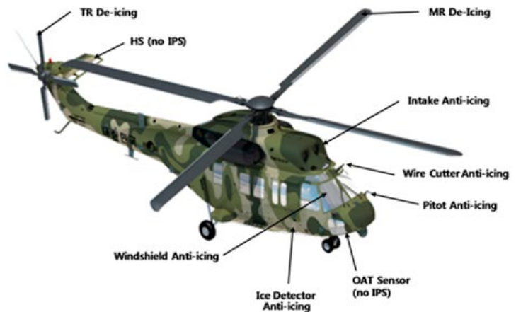
Figure 2. KUH-1 ice protection system. Overview of ice protected systems installed on test aircraft.
