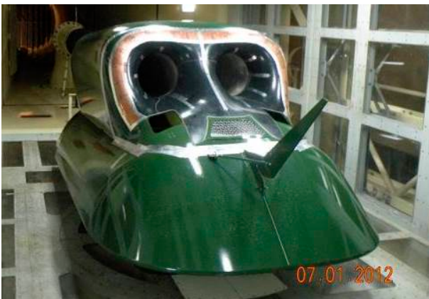
Figure 3. KUH-1 engine air intake wind tunnel model. Full-scale engine air intake wind tunnel model tested in the CIRA icing wind tunnel.
