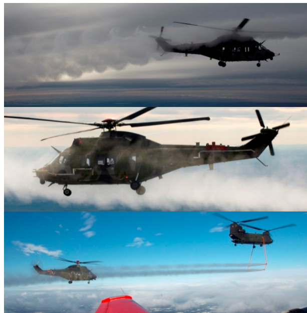
Figure 9. HISS spray immersion position. Relative vertical positions selected for rotor, upper fuselage and lower fuselage icing.
