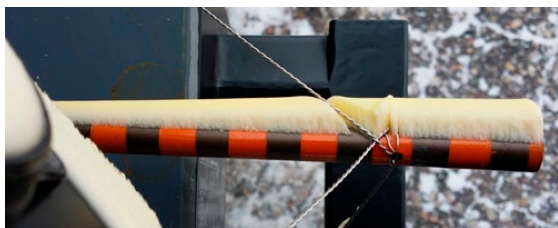
Figure 11. Ice thickness distribution on fuselage-mounted icing blade. Ice thickness documented on the ground after a 100 km HISS spray exposure at -21.1^{\circ}\text{C} ambient temperature, 0.53\text{ g/m}^3 liquid water content and 19.3\text{ }\mu\text{m} median volume diameter. Marker width = 1 cm.
