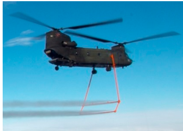
Figure 5. Helicopter Icing Spray System. RTC HISS tanker with spray boom deployed.
