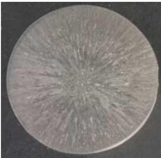
Figure 1. Optical macrograph of ABB-23 Ø16 mm cast bar structure.
