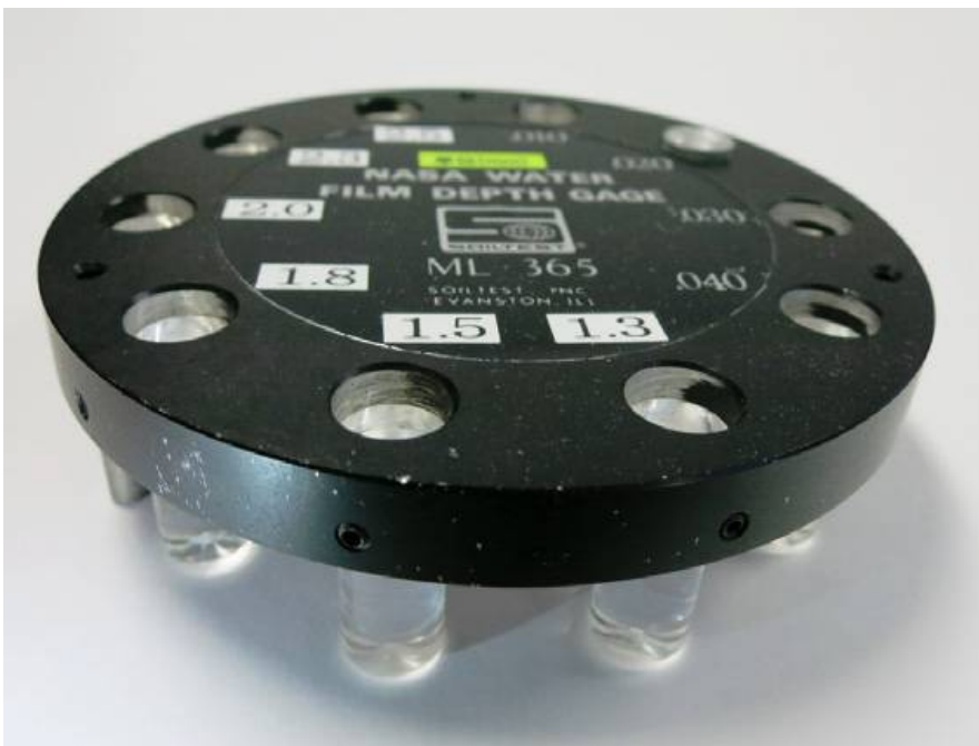
Figure 2: NASA water film depth gauge.
