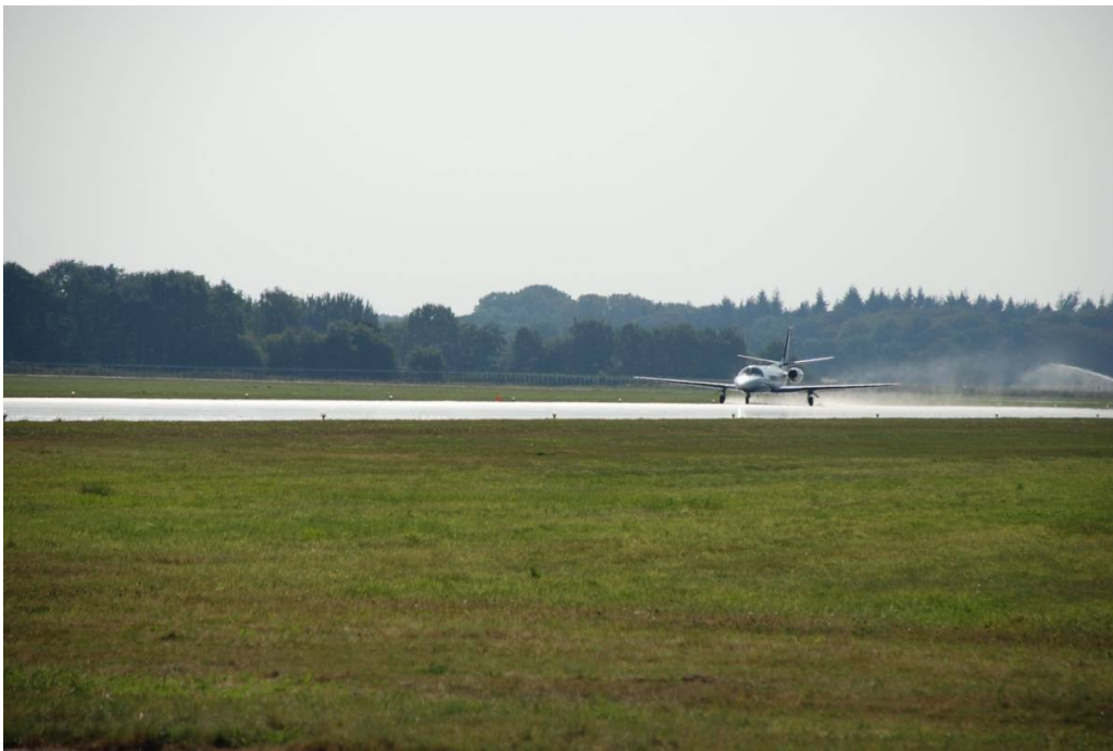
Figure 6: Aircraft braking at the beginning of the wet test section.
