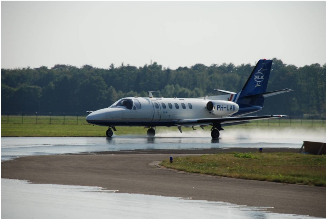
Figure 7: Aircraft braking at the end of the wet section.
