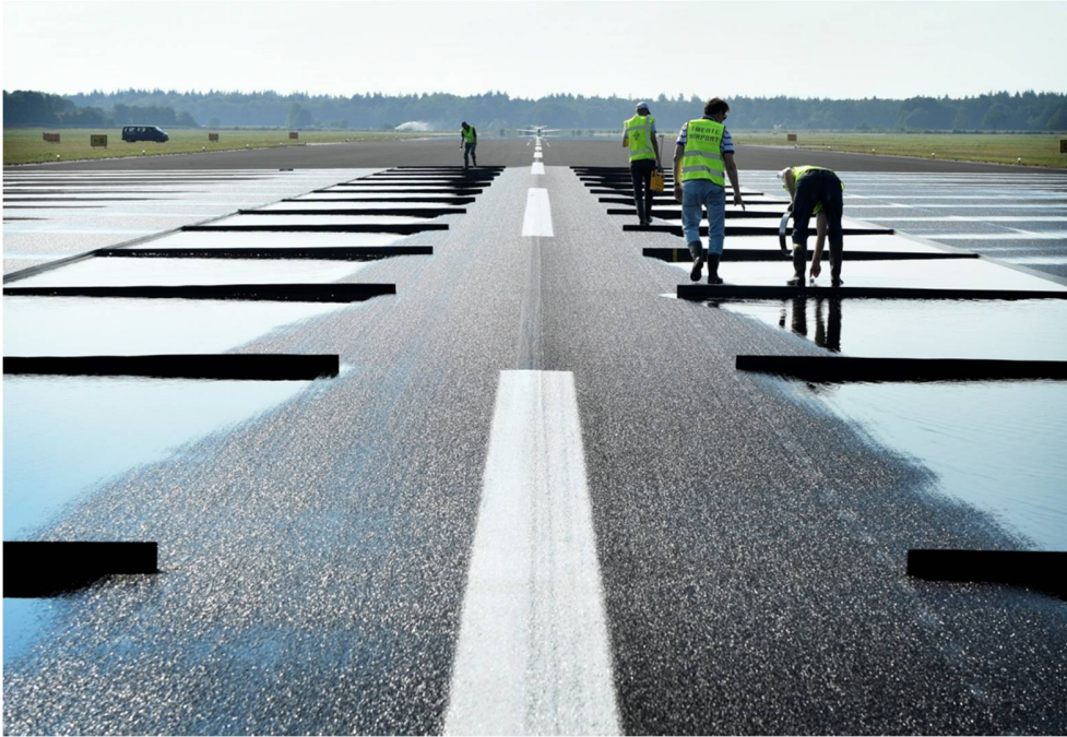
Figure 15: Example of measuring water depth level in each section.
