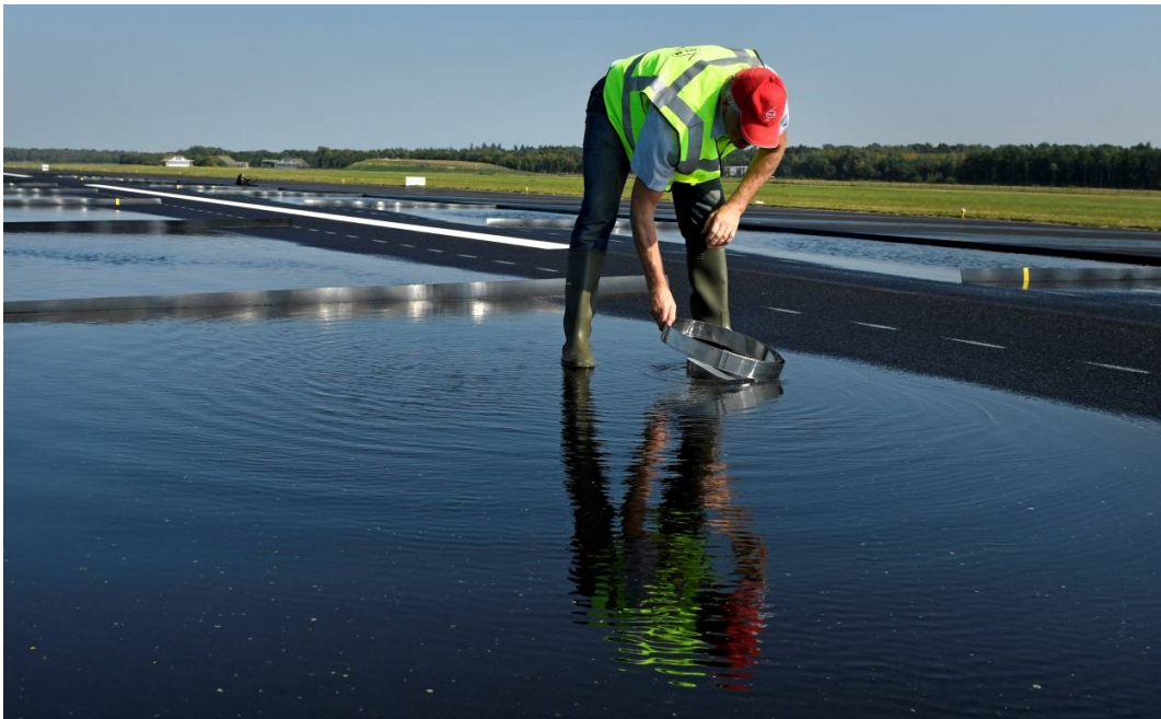
Figure 18: Measuring of water depth using a metal ring around the water depth gauge.
