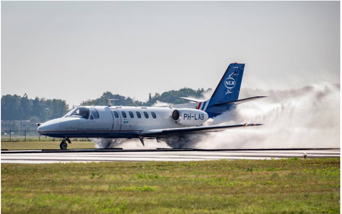
Figure 22: Cessna Citation test aircraft running through the water pond.
