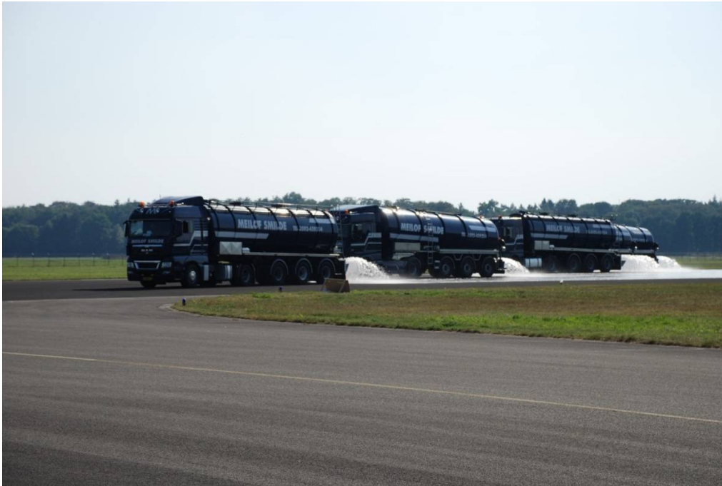
Figure 5: Wetting of the runway using water tank trucks.
