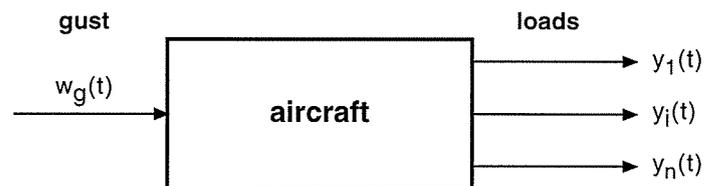
Suppose the input gust  $w_g(t)$  is a stationary random process  $\underline{w}_g(t)$  having a Gaussian probability distribution with standard deviation  $\sigma_w$  and normalized power spectral density function  $\Phi_w^n(\omega)$ .
