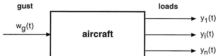
The "input" gust  $w_g(t)$  induces "output" gust loads  $\bar{y}(t) = \{y_1(t), y_2(t) \dots y_n(t)\}$ .
