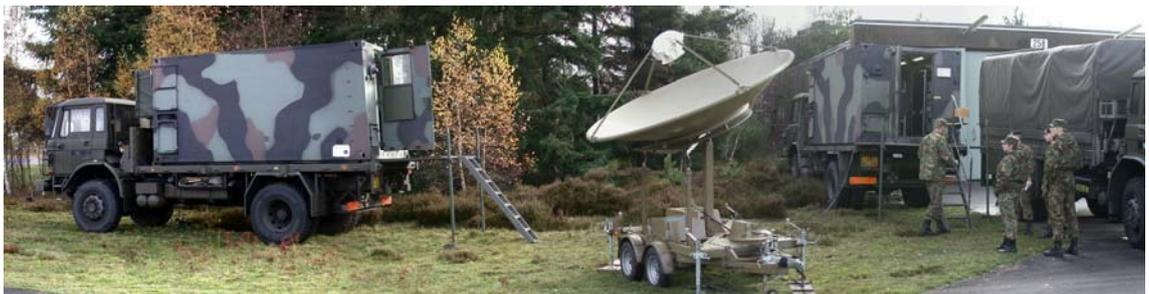
*Fig. 1 RAPIDS mobile ground receiving station deployed during exercise Low Lands*
