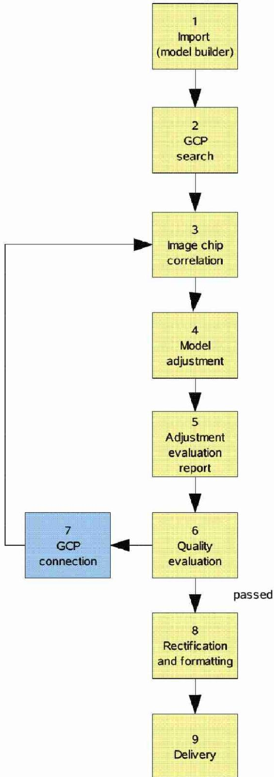
Fig. 4 Flow diagram for automatic ortho-rectification
